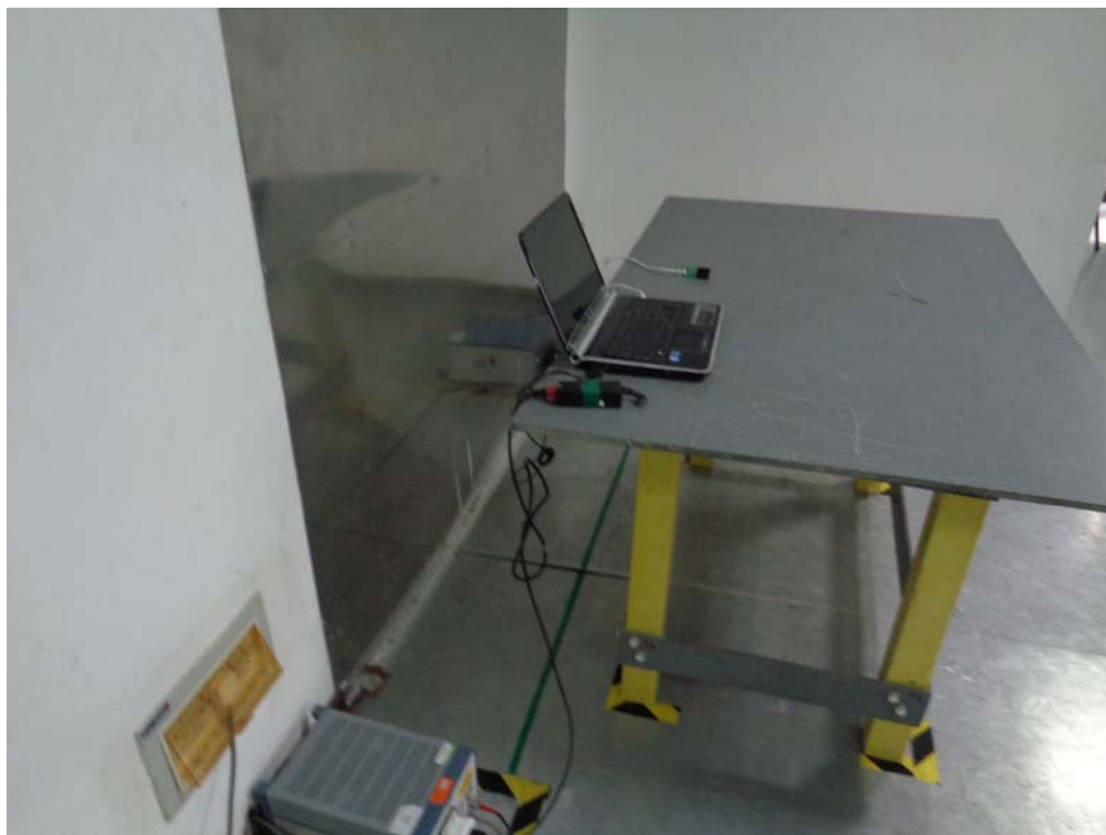
Conducted Emissions Test Setup Side View
