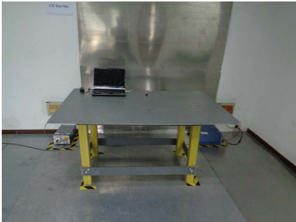
Conducted Emissions Test Setup Front View
