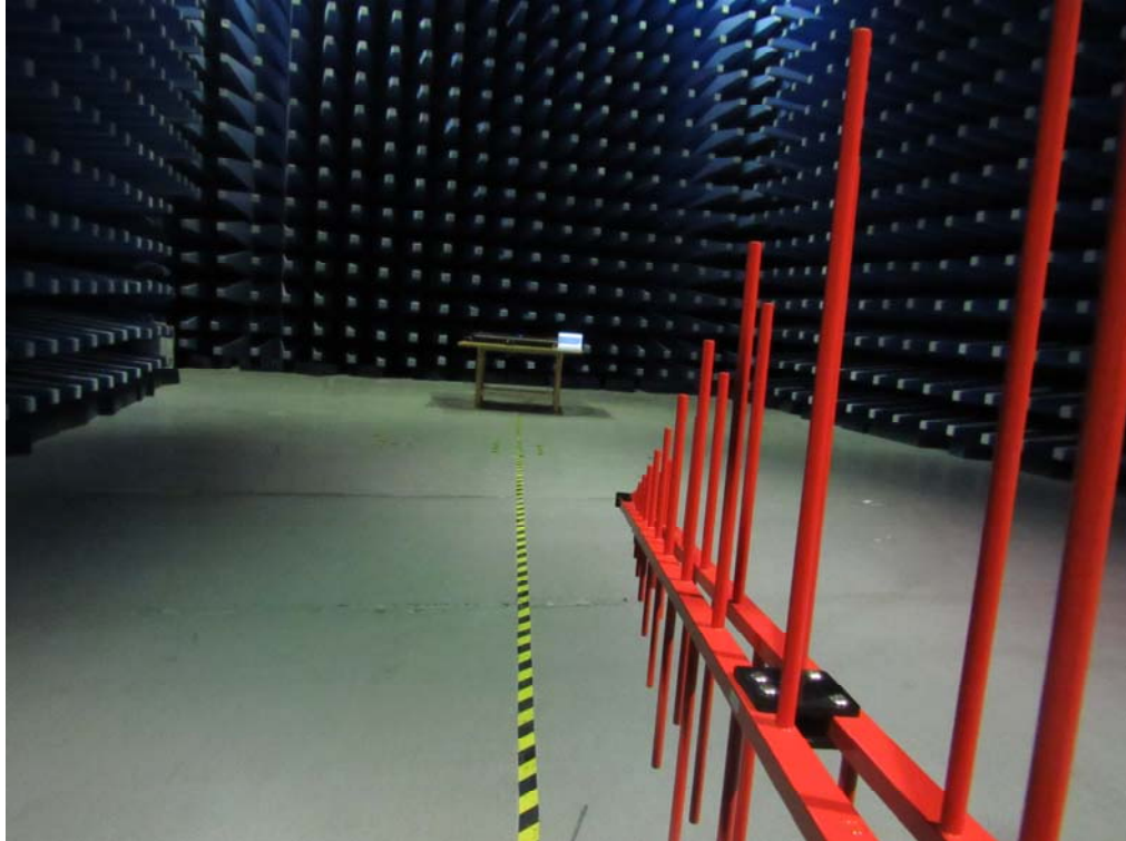
Radiated Emissions Setup Below 1GHz Front View
