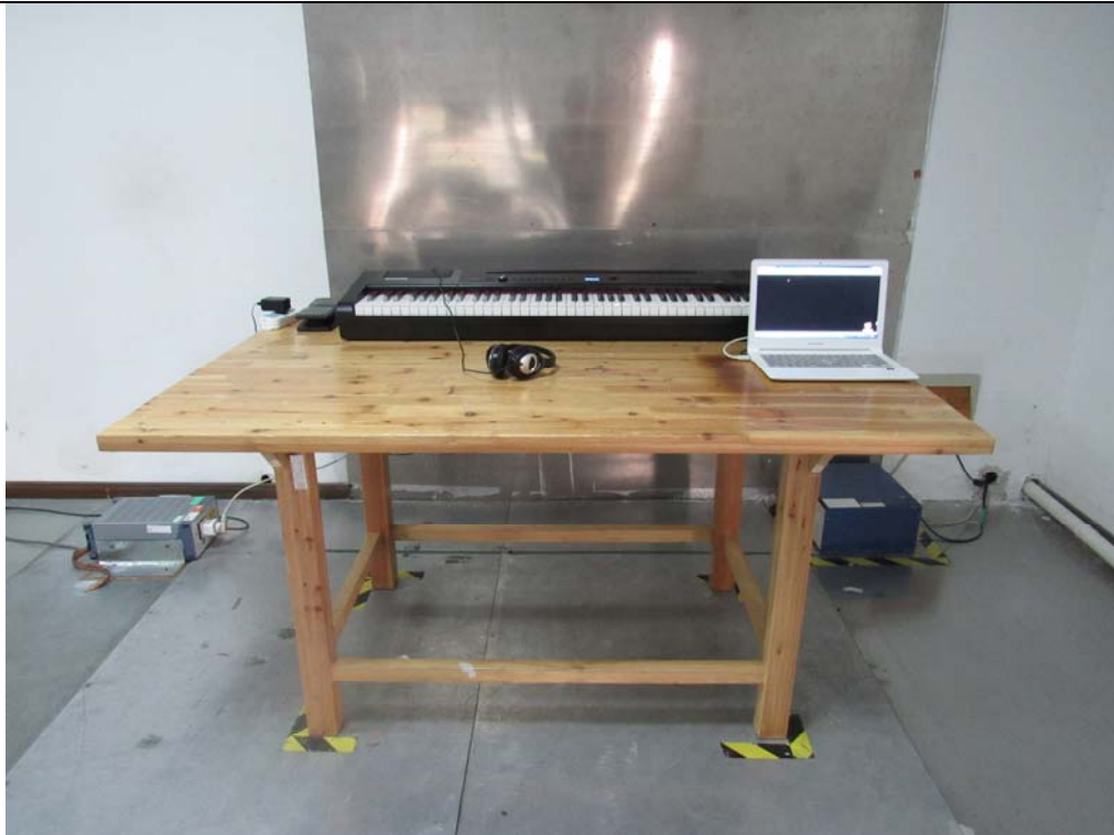
Conducted Emissions Setup Front View
