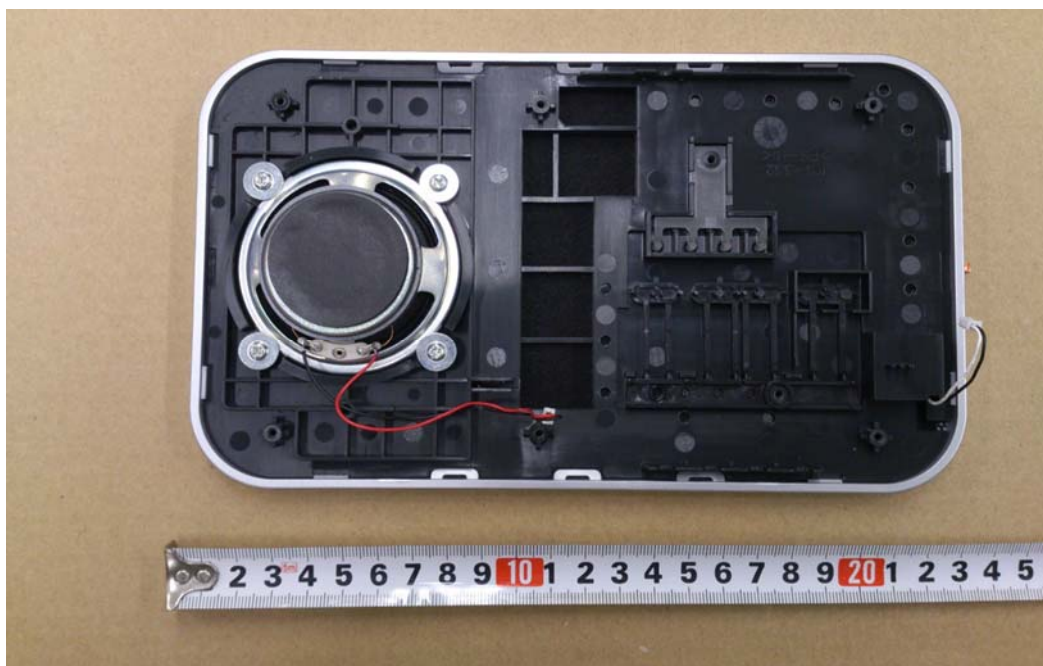
R-Talk 800EX Inside the product(There is not mounting board)
