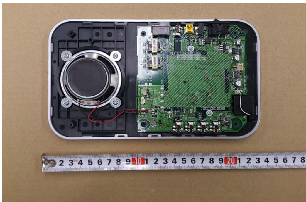
R-Talk 800EX Inside the product(There is mounting board)
