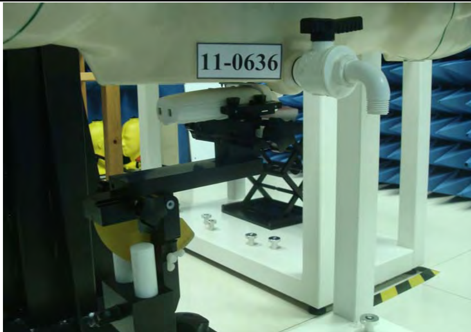
Figure 7. Body SAR Test Setup (Flat Section)
