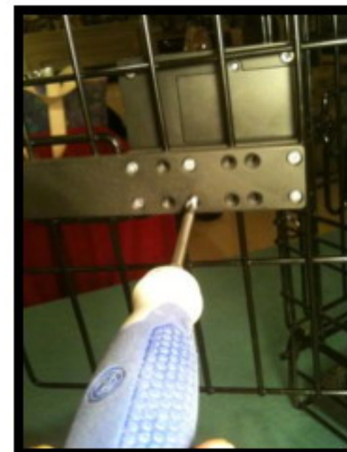
Figure 6. Install screws in the 4 outer screw holes and any other two holes loosely.
