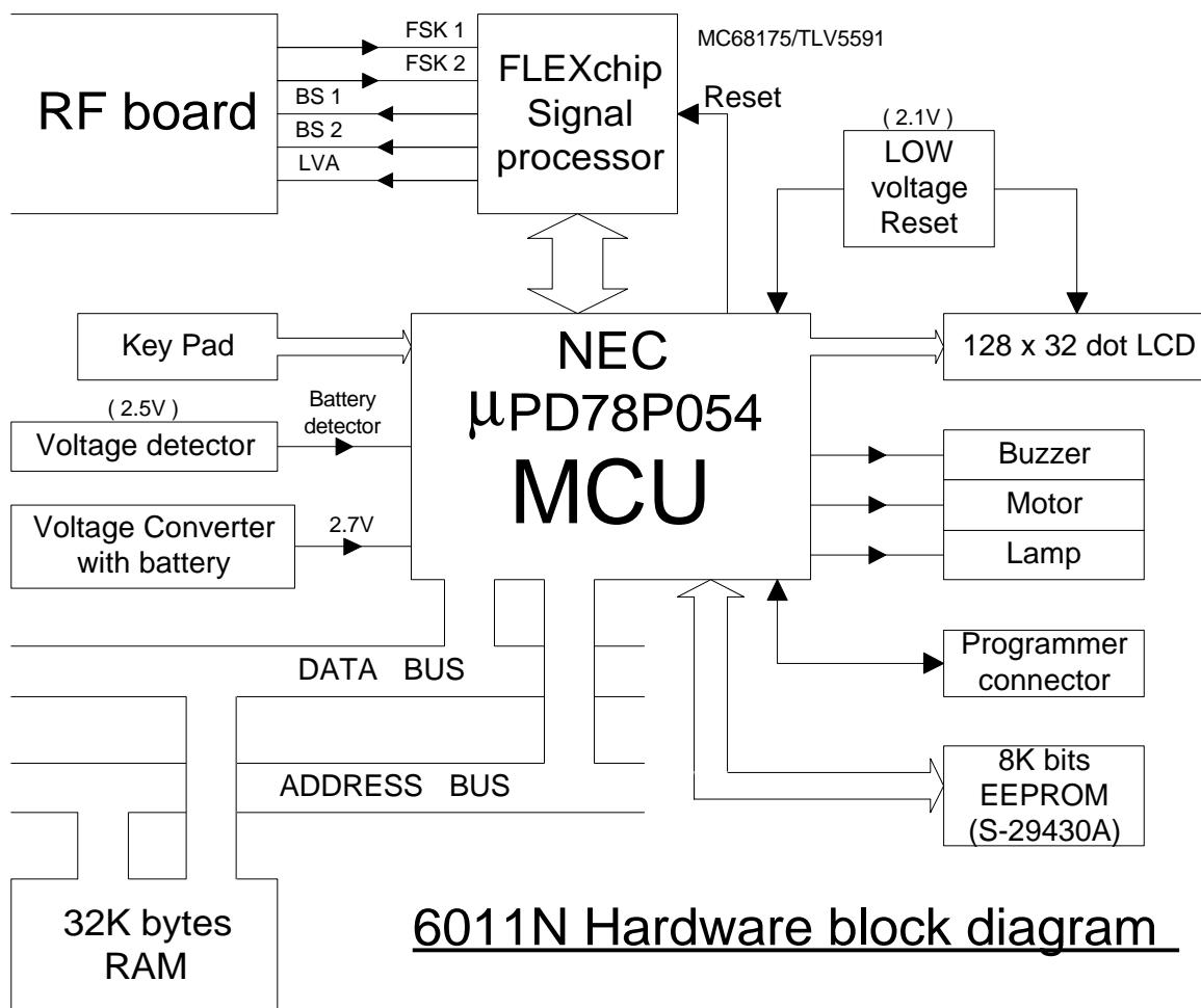
Figure 1: Block diagram of 6011N digital architecture.
