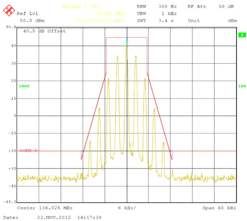
**Emission Mask- Channel – Type D (low power level)**
