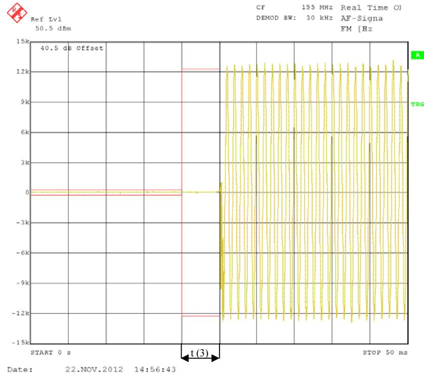
**Turn on –Middle Channel (low power level)**
