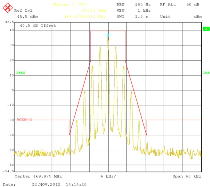
**VHF – low channel:****Occupied Bandwidth**
