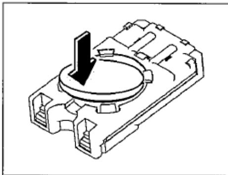
4. Put new battery on the module and push down it into the position.
