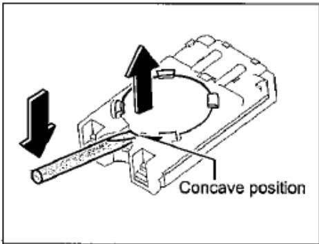
3. Insert the screwdriver (-) to the concave portion, then remove the battery.
