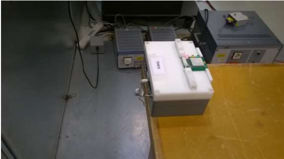
Figure 7 - Conducted Emissions Test Setup
