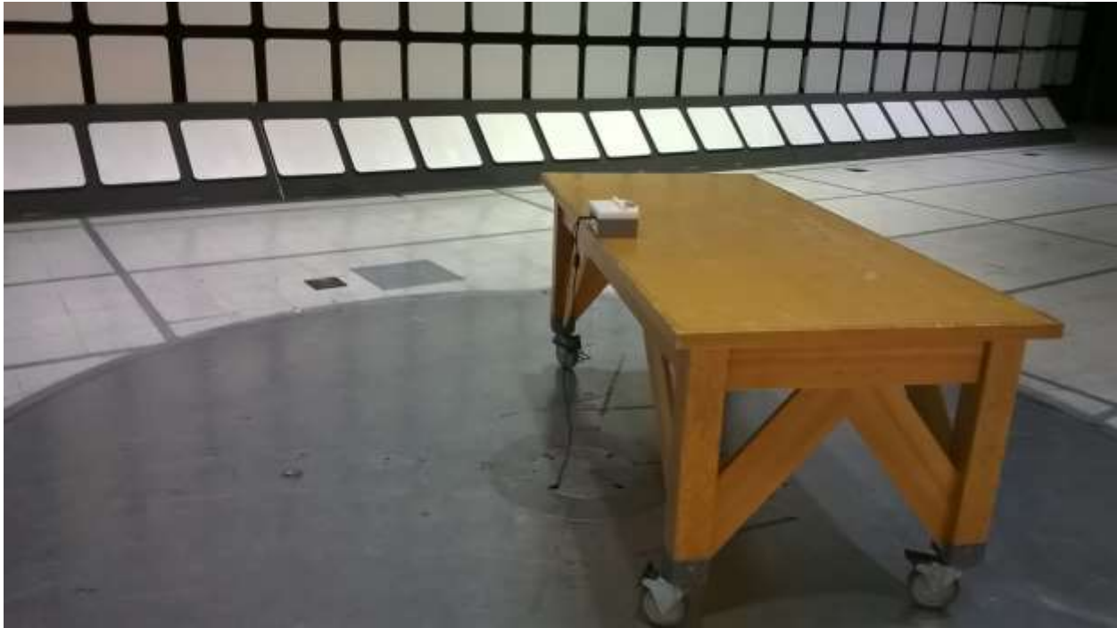
Figure 5 - Radiated emissions test setup, 30MHz - 1GHz
