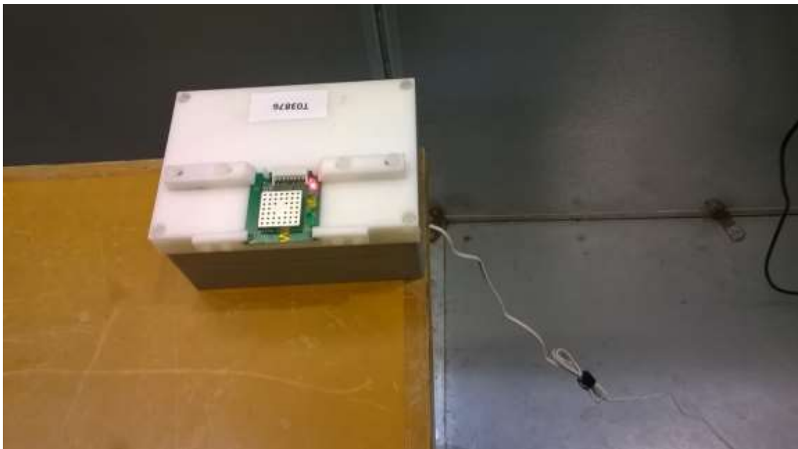
Figure 8 - Conducted Emissions Test Setup
