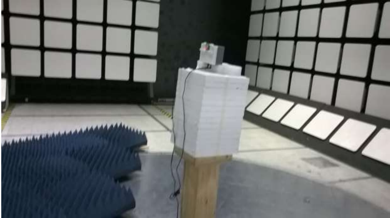
Figure 3 - Radiated emissions test setup, 1GHz - 25GHz
