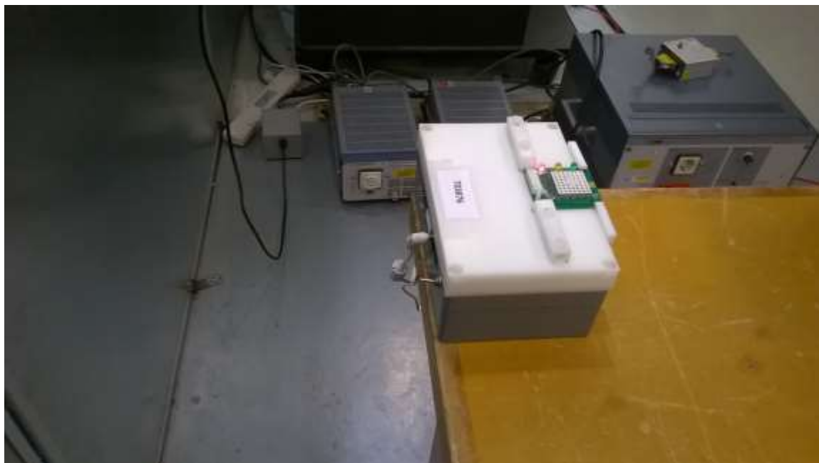
Figure 29 - Conducted Emissions Test Setup
