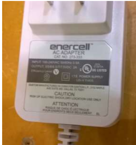
Figure 28 - AC/DC Power Used for Conducted Emissions
