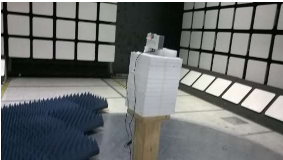
Figure 26 - Radiated Emissions Test Setup
