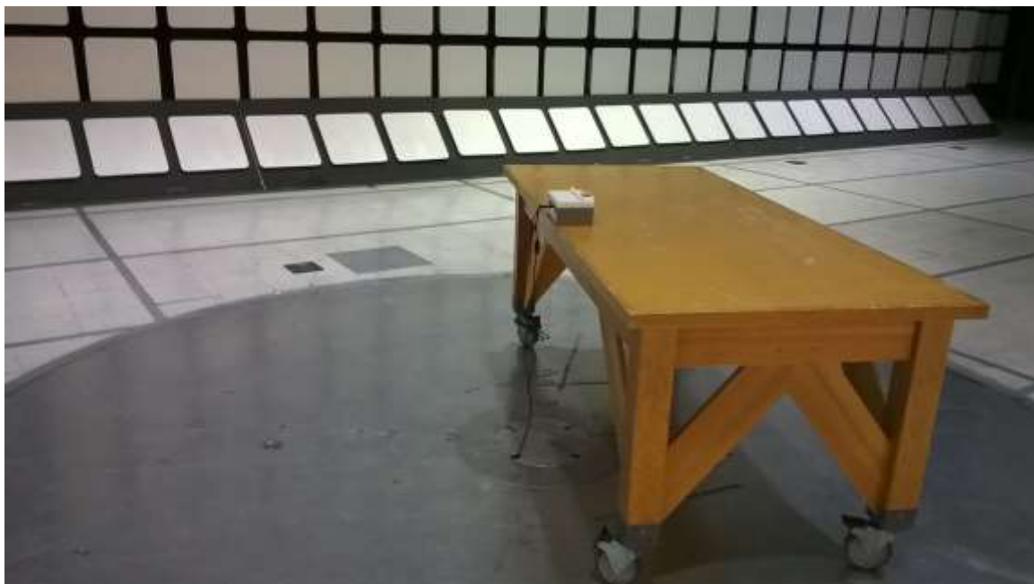
Figure 25 - Radiated Emissions Test Setup
