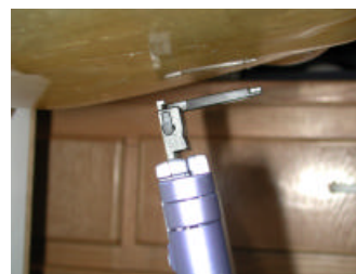
Fig. 9 Body SAR Test Setup
