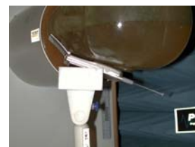
Fig. 14 Head SAR Test Setup
