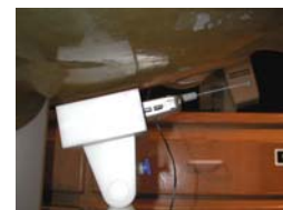
Fig. 15 Body SAR Test Setup
