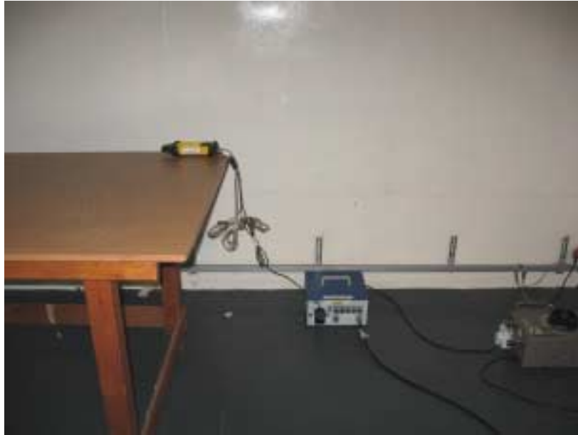
Photograph No.5 Setup for conducted emission measurements on the power lines
