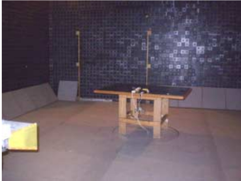
Photograph No.7 Setup for radiated emission measurements in the anechoic chamber above 1000 MHz
