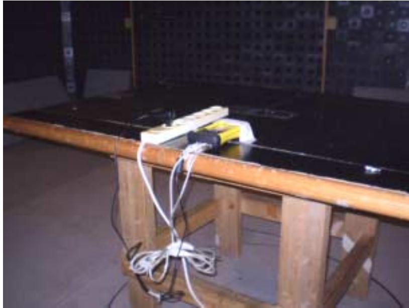
Photograph No.8 Setup for radiated emission measurements in the anechoic chamber, close view
