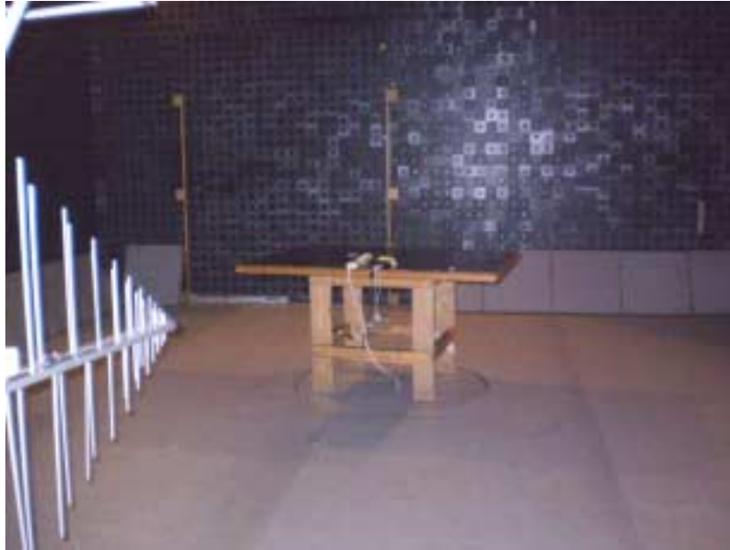
Photograph No.6 Setup for radiated emission measurements in the anechoic chamber from 30 to 1000 MHz
