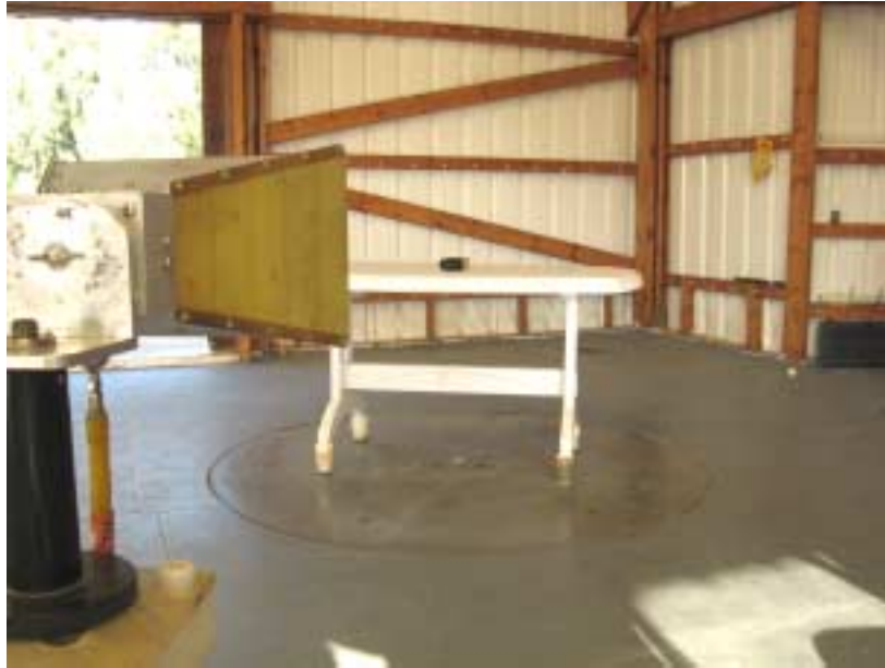
Photograph No.3 Setup for spurious emission measurements at the OATS above 1000 MHz
