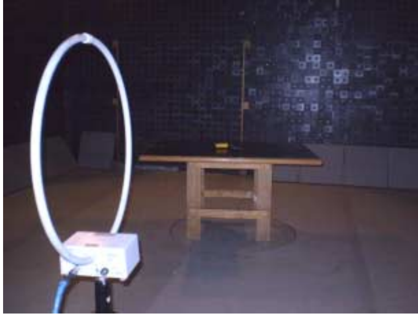
Photograph No.1 Setup for spurious emission and occupied bandwidth measurements in the anechoic chamber below 30 MHz
