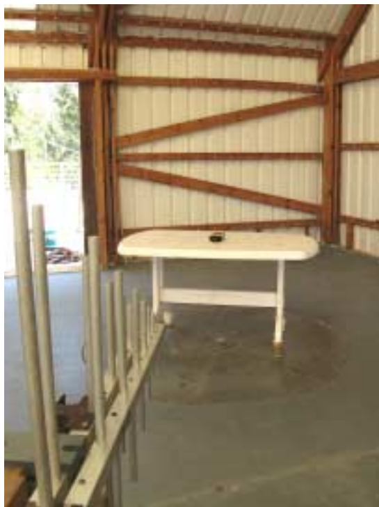
Photograph No.2 Setup for fundamental and spurious emission measurements at the OATS from 30 to 1000 MHz
