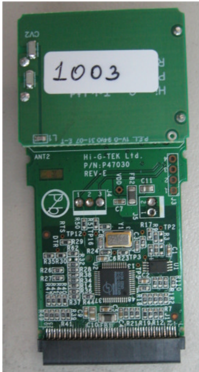
Photograph No4 Master Handheld Terminal PCB second side view
