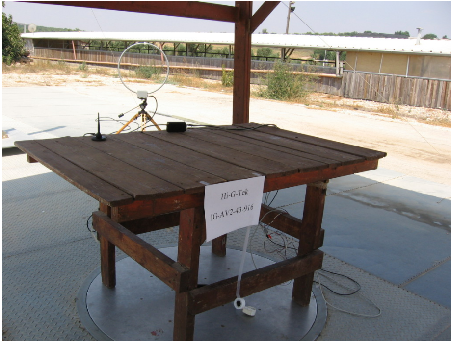
Figure 6. Radiated Emission Test 9kHz-30MHz
