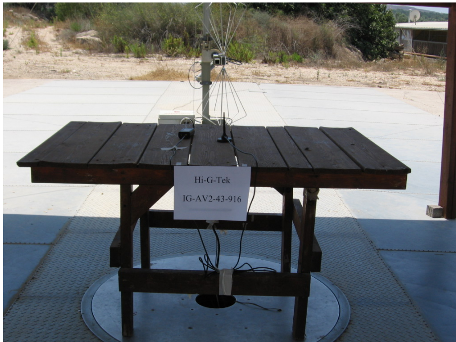
Figure 7. Radiated Emission Test 30MHz-9.2GHz
