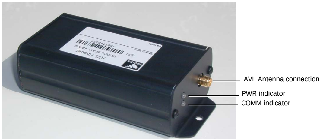
Figure 1-2. AVL Reader Antenna Connection Side
