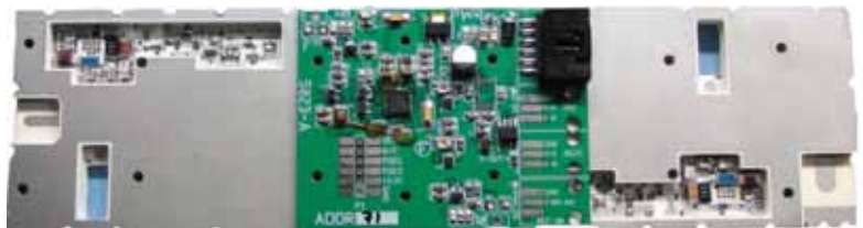
ODC / UDCC Assembly with cover removed
