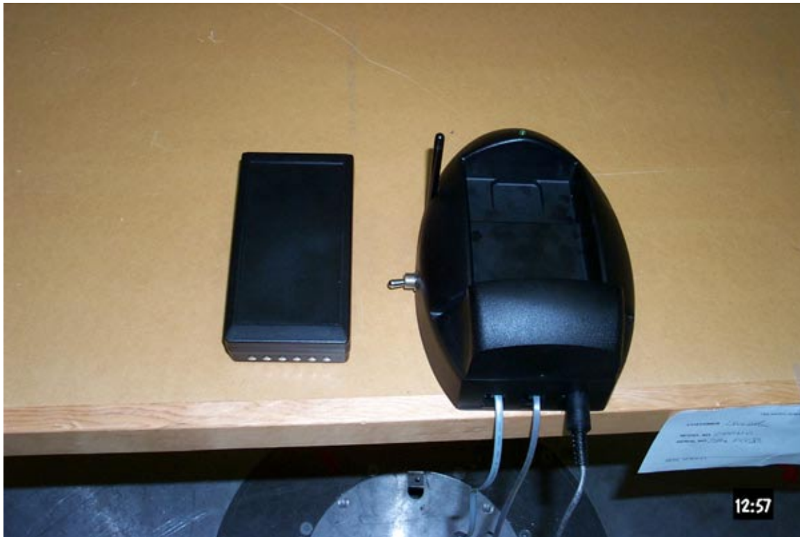
Figure 15 PTU and base (switch on side for testing)
