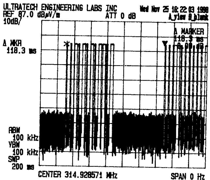
$$\text{DUTY CYCLE} = \frac{6 \times 1.14 + 6 \times 3.43}{100} = 0.2742 \text{ or } -11.2 \text{ dB}$$
