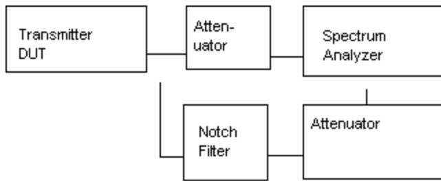
Method of Measuring Conducted Spurious Emissions
