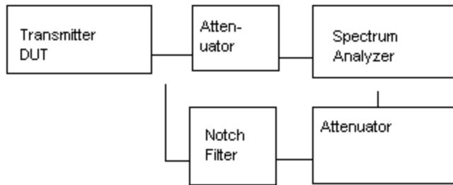
Method of Measuring Conducted Spurious Emissions
