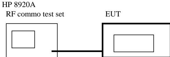
FM modulation deviation was measured at different frequencies at a constant input of 2 VRMS. Maximum deviation was measured for audio input at 80 Hz.
