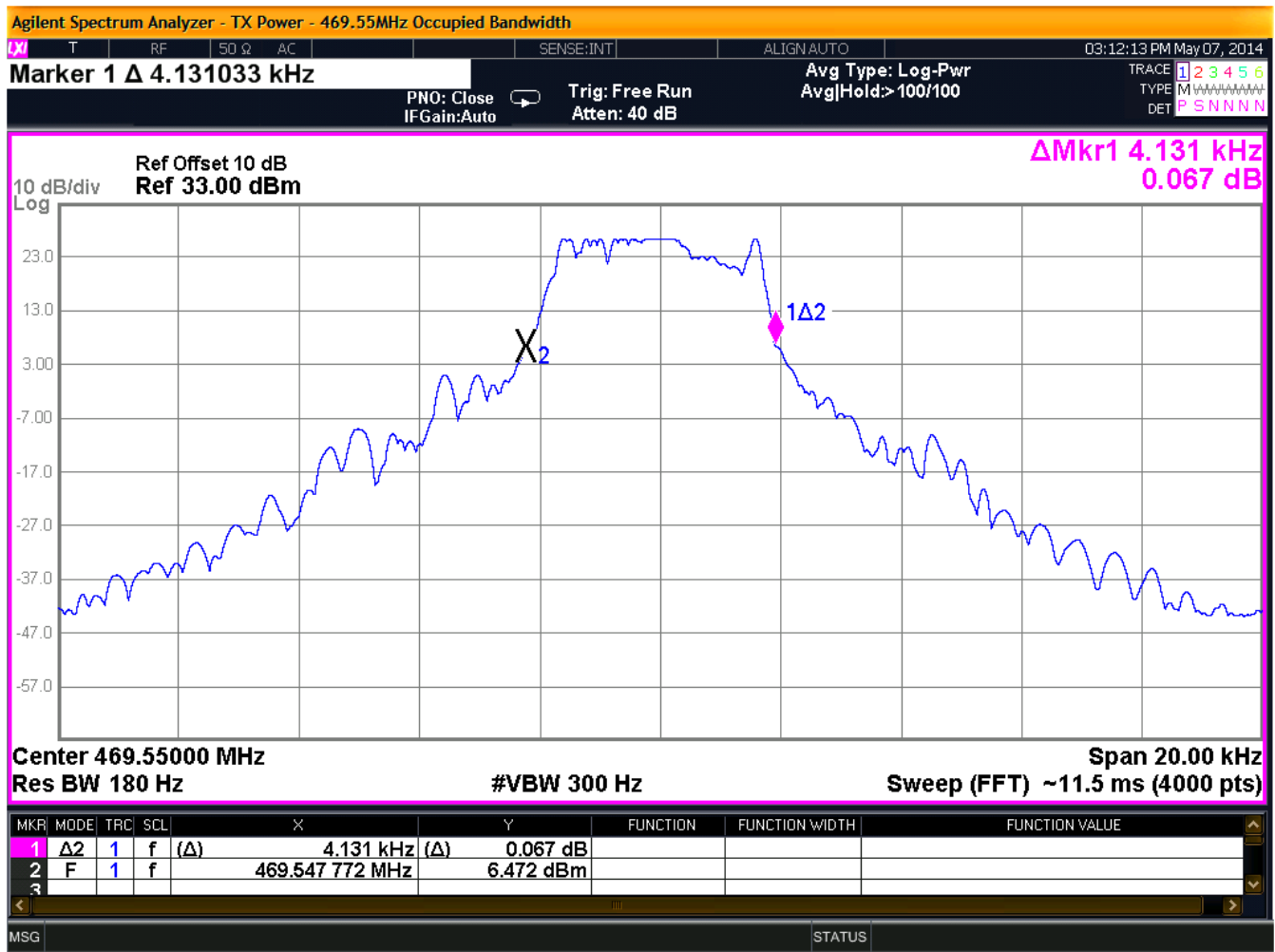
Figure 6: High Channel Occupied Bandwidth @469.55MHz
