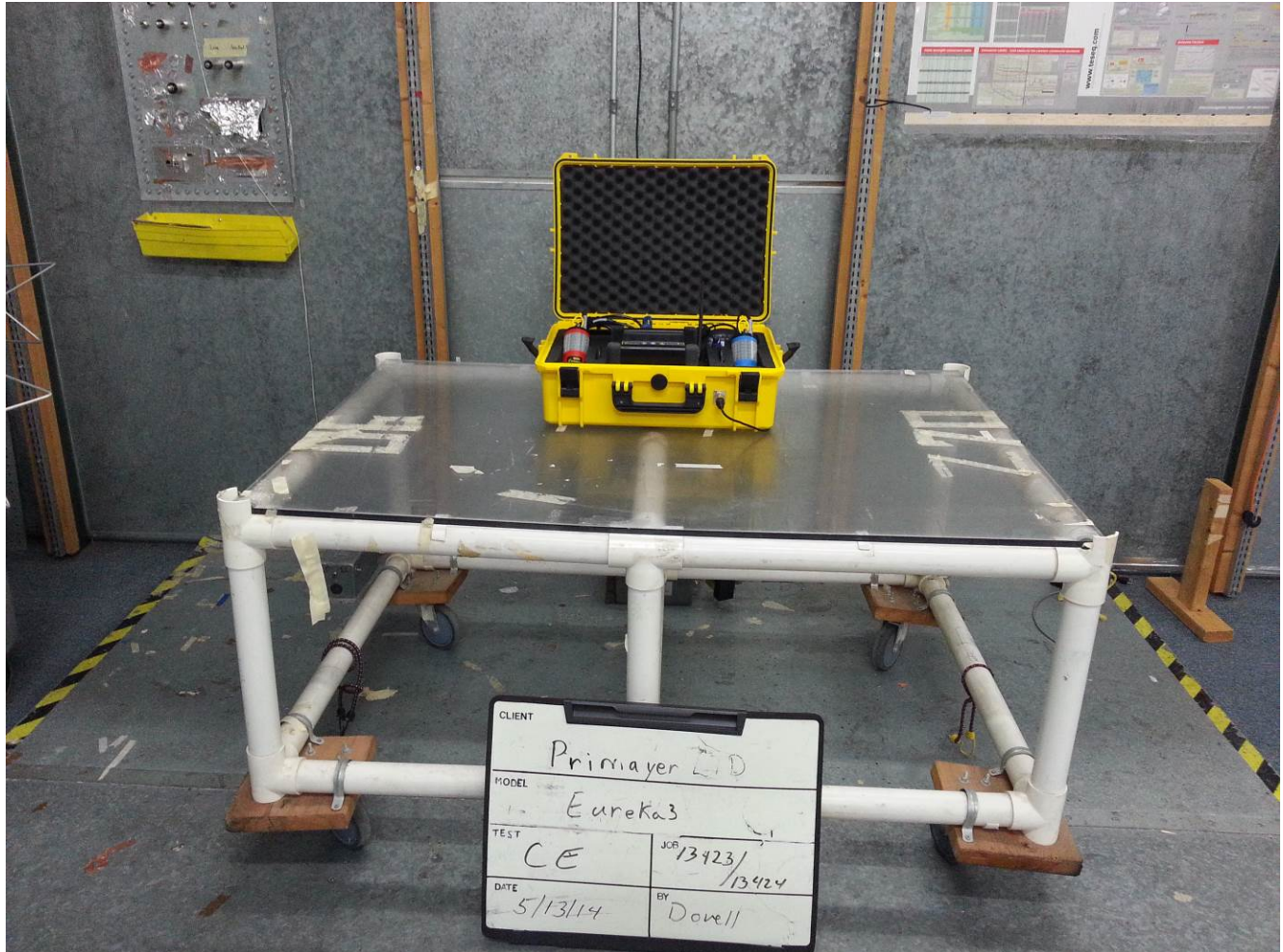
Photograph 4: Conducted Emission Test Configuration, Front
