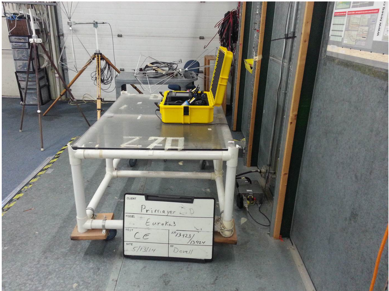
Photograph 5: Conducted Emission Test Configuration, Side
