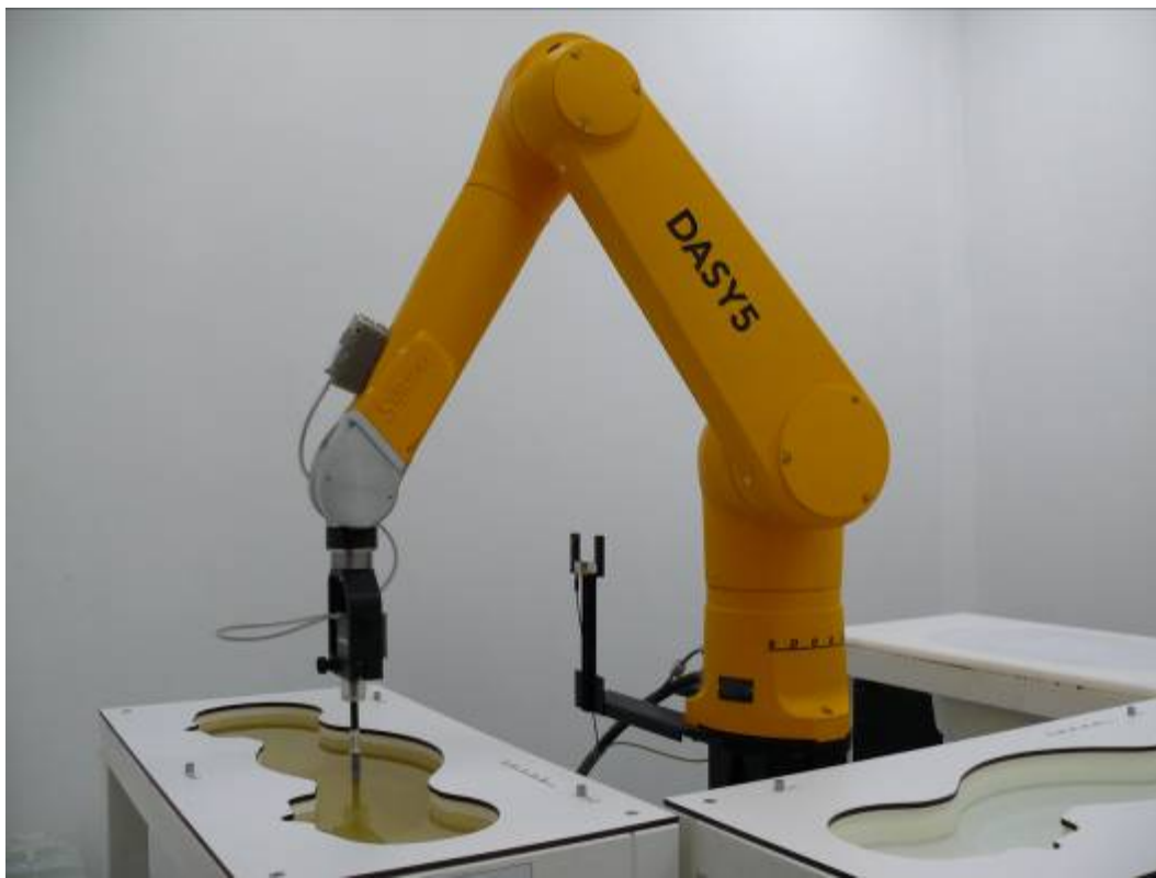
Picture 1: Specific Absorption Rate Test Layout
