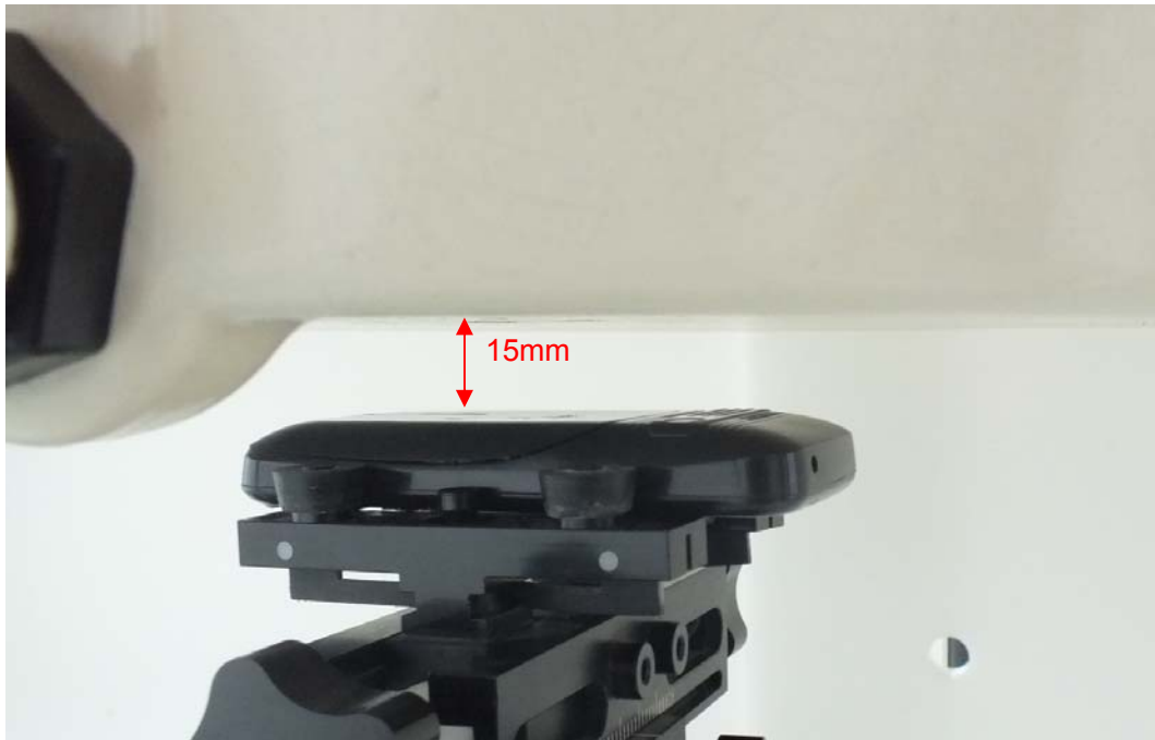
Picture 11: Back Side, the distance from handset to the bottom of the Phantom is 15mm
