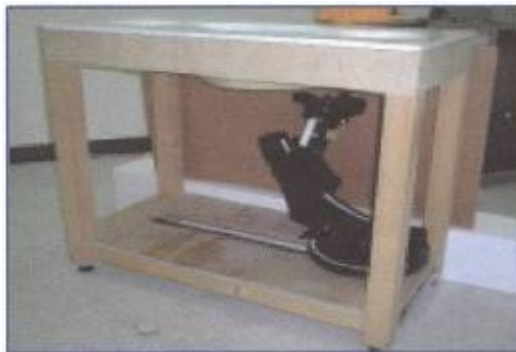
Figure 5 Generic Twin Phantom
