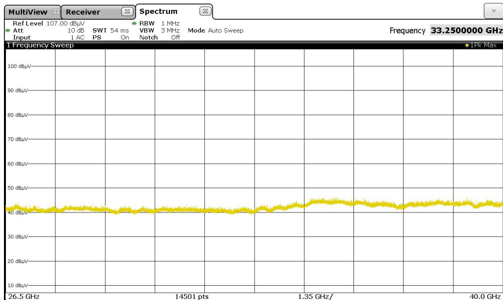
172171_9.jpeg: Spurious emissions from 26.5 GHz to 40 GHz:
