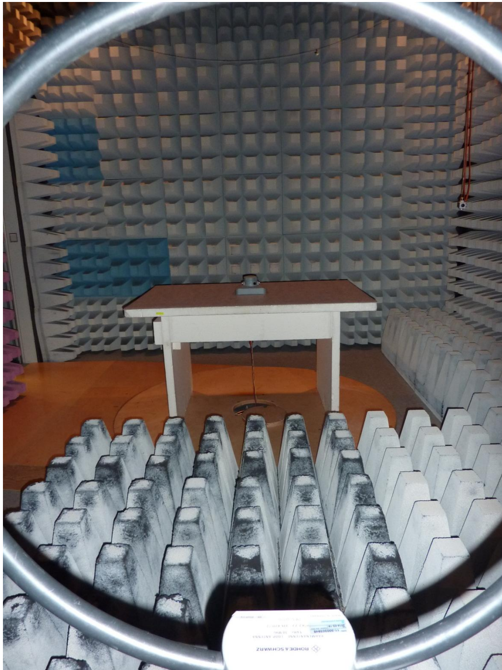
143563_6.JPG: RLS, test set-up fully anechoic chamber
