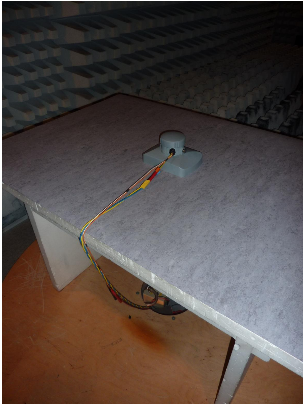
143563_7.JPG: RLS, test set-up fully anechoic chamber (normal position)
