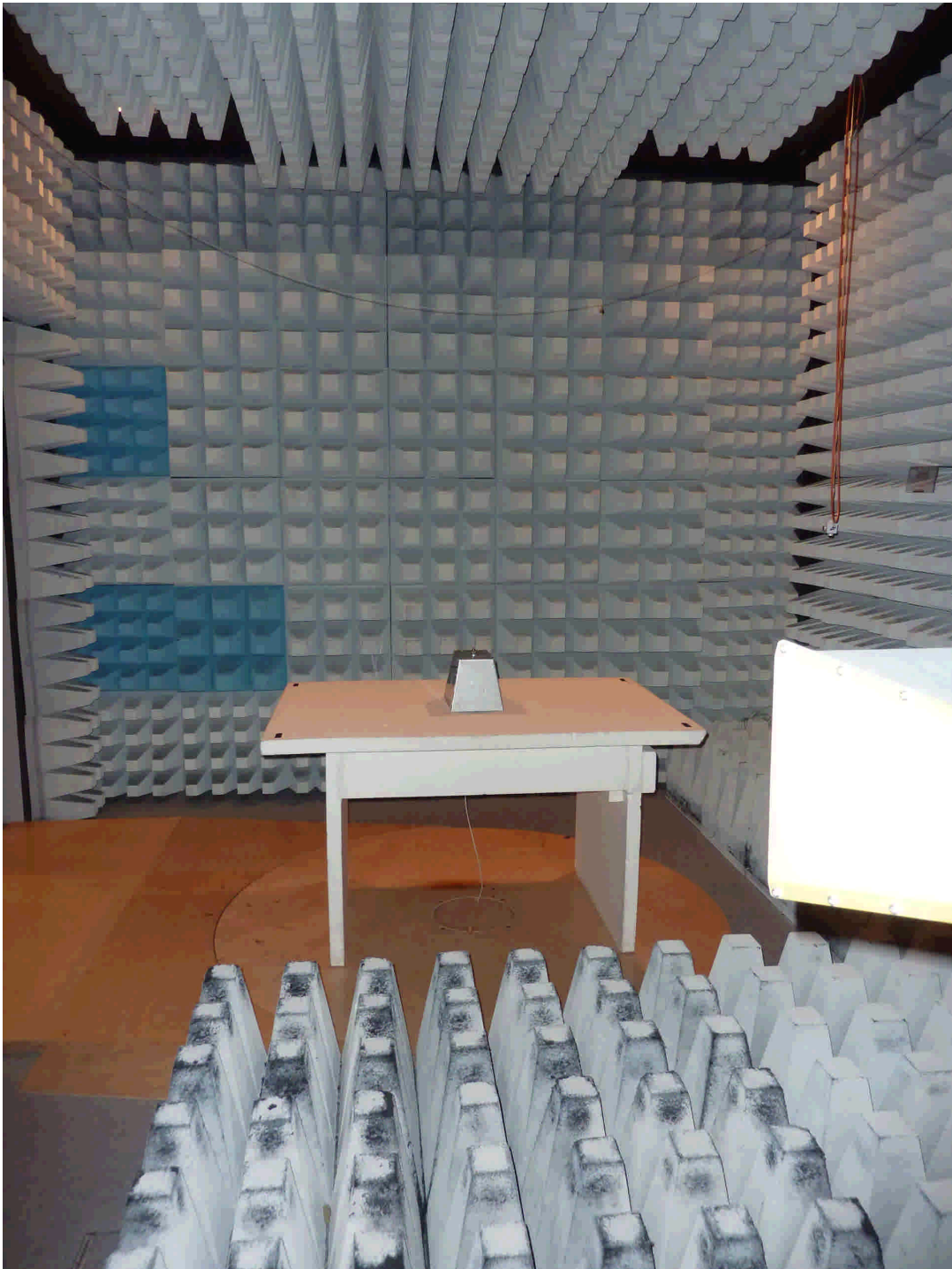
110464_6.jpg RLS, test set-up fully anechoic chamber
