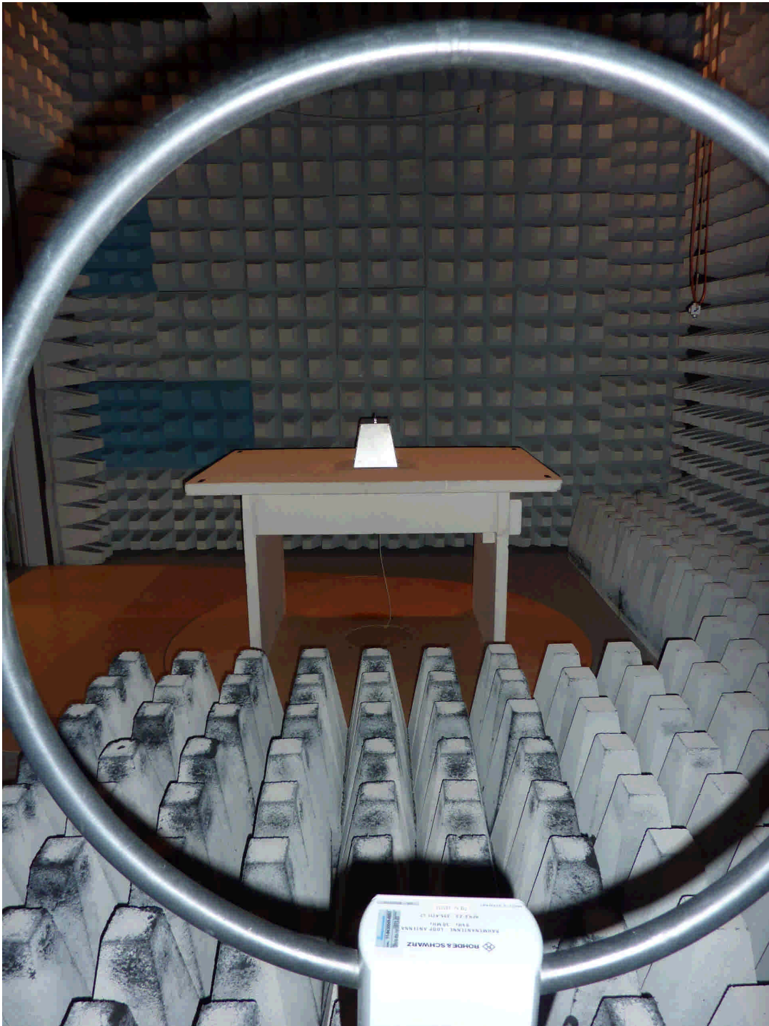
110464_5.jpg RLS, test set-up fully anechoic chamber
