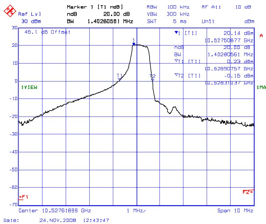
**5.5.5.3. Plot#3 - Antenna #3 Configuration: 20dB Bandwidth**
