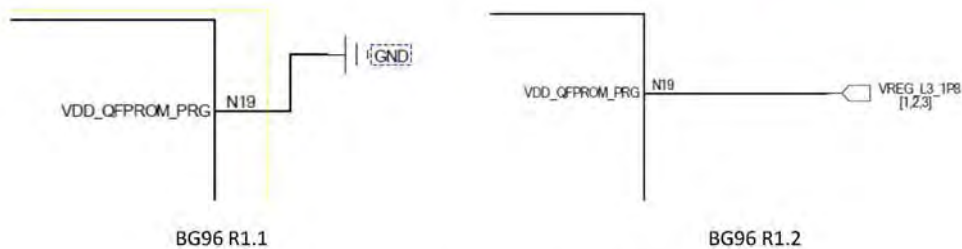
Figure 1: Schematic Designs of BG96 R1.1 and R1.2
