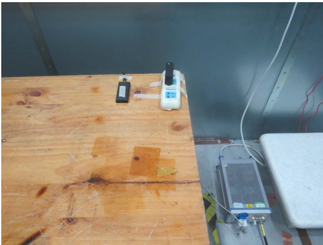
Picture 2 Conducted Emission Test Setup
