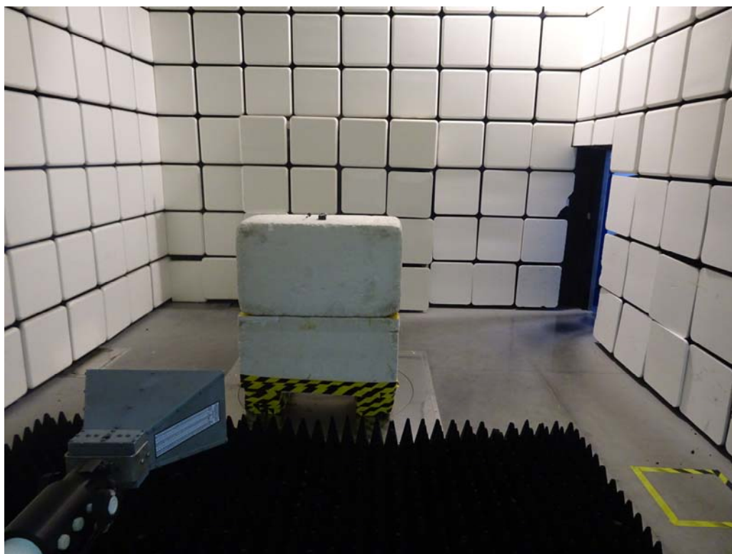
Picture 1: Radiated Spurious Emissions Test setup
