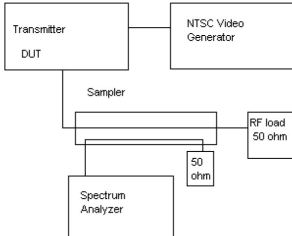
2.1051 Spurious emissions at antenna terminals (conducted):
