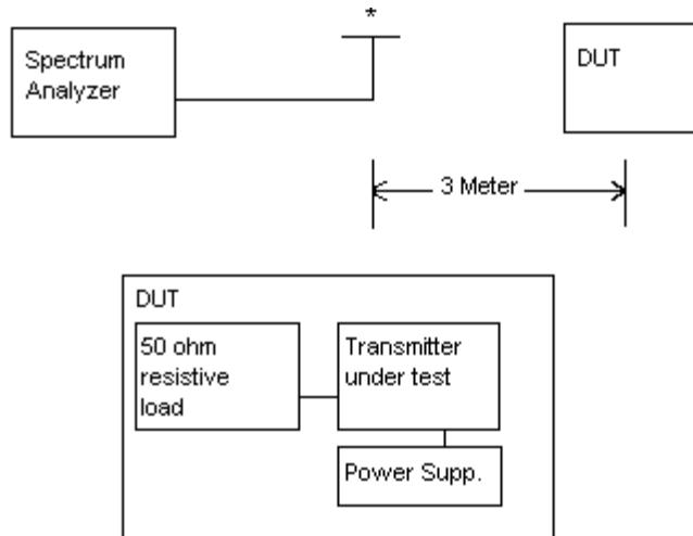
(\*) Is a tuned calibrated antenna which may be raised from 1 to 4 meters above ground and changed in polarization from vertical to horizontal.
