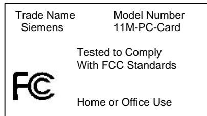
The above label will be used on the PCMCIA card to meet the DOC label requirements. It will be located on a flat surface along the edge on the bottom.
