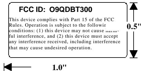
Specifications: Text is black in color and is left justified. Labels are printed in indelible ink on permanent adhesive backing and shall be affixed at a conspicuous location on the EUT.
