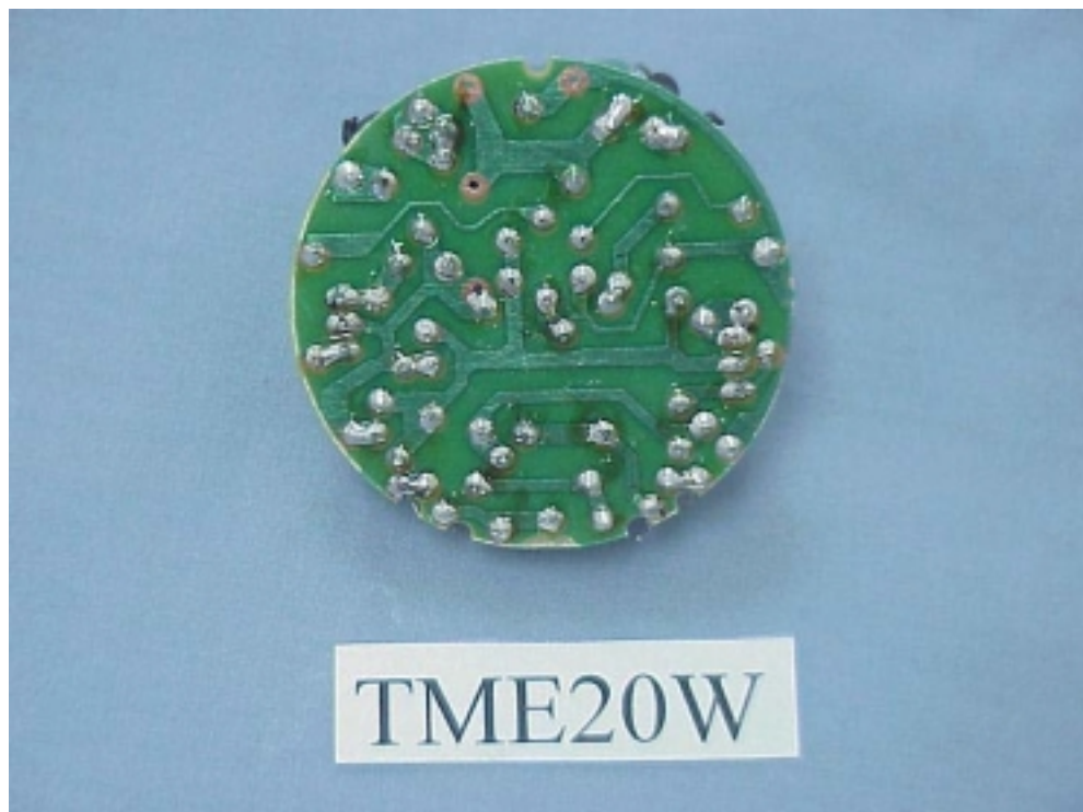
Figure 5 ENERGY SAVING LAMP (M/N: TME20W) MAIN BOARD (SOLDERED SIDE)
