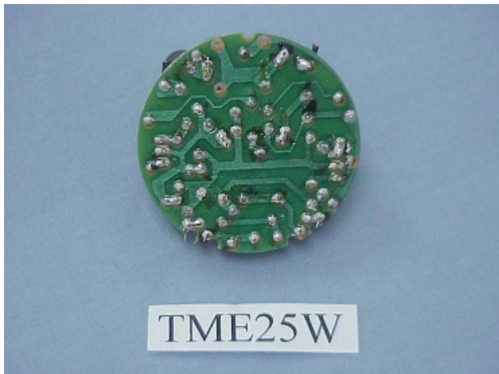
Figure 7 ENERGY SAVING LAMP (M/N: TME25W) MAIN BOARD (SOLDERED SIDE)
