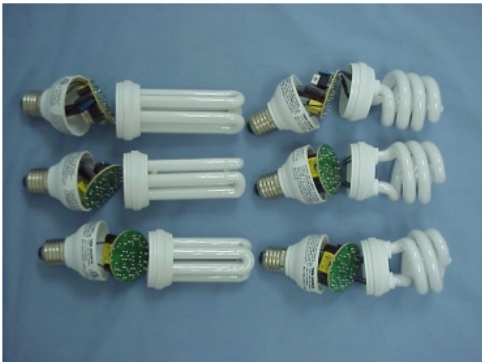
Figure 2 Energy Saving Lamp (M/N: TME15W, TME20W, TME25W) Cover Removed
