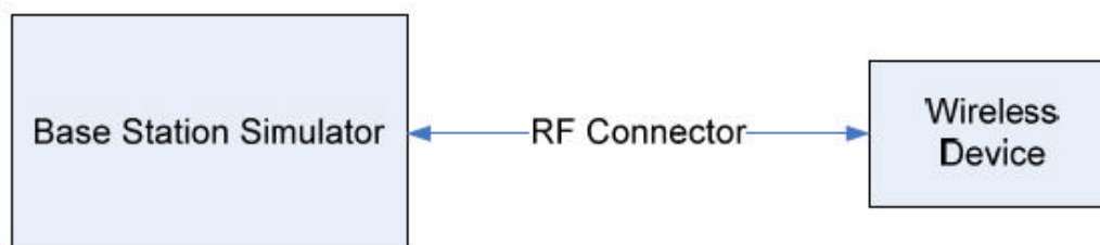
Figure 6-1. CDMA Conducted Power Test Setup Diagram
