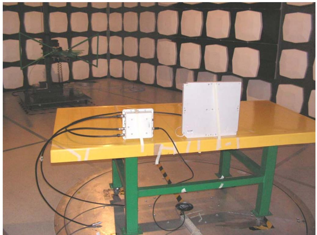
Ant. 2 for Test Configuration: above 1GHz
