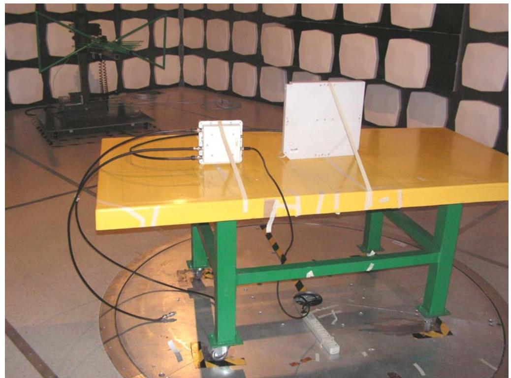
Ant. 3 for Test Configuration: 9KHz~1GHz
