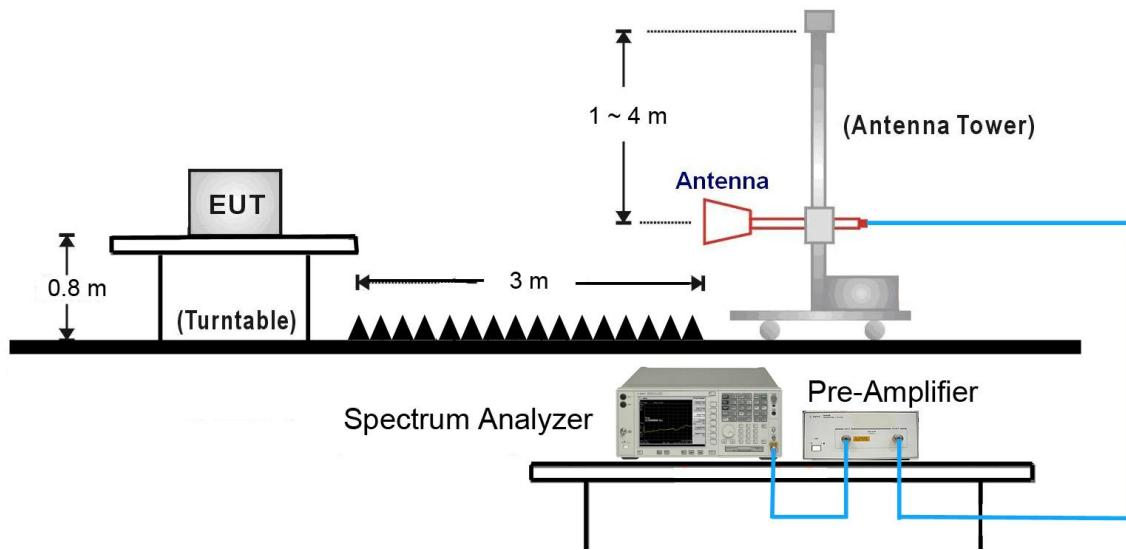
18GHz ~25GHz Test Setup:
