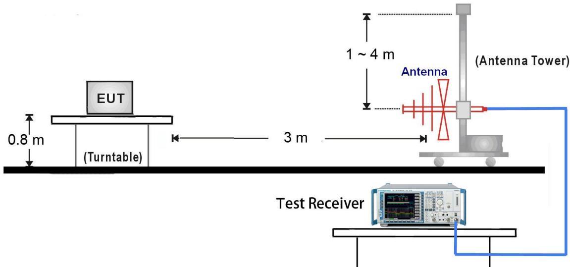
1GHz ~ 18GHz Test Setup:
