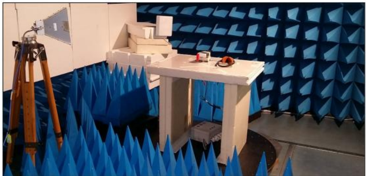
Test setup in anechoic chamber
