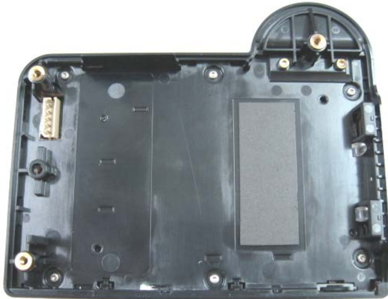
Photograph No.6 Data recorder battery space
