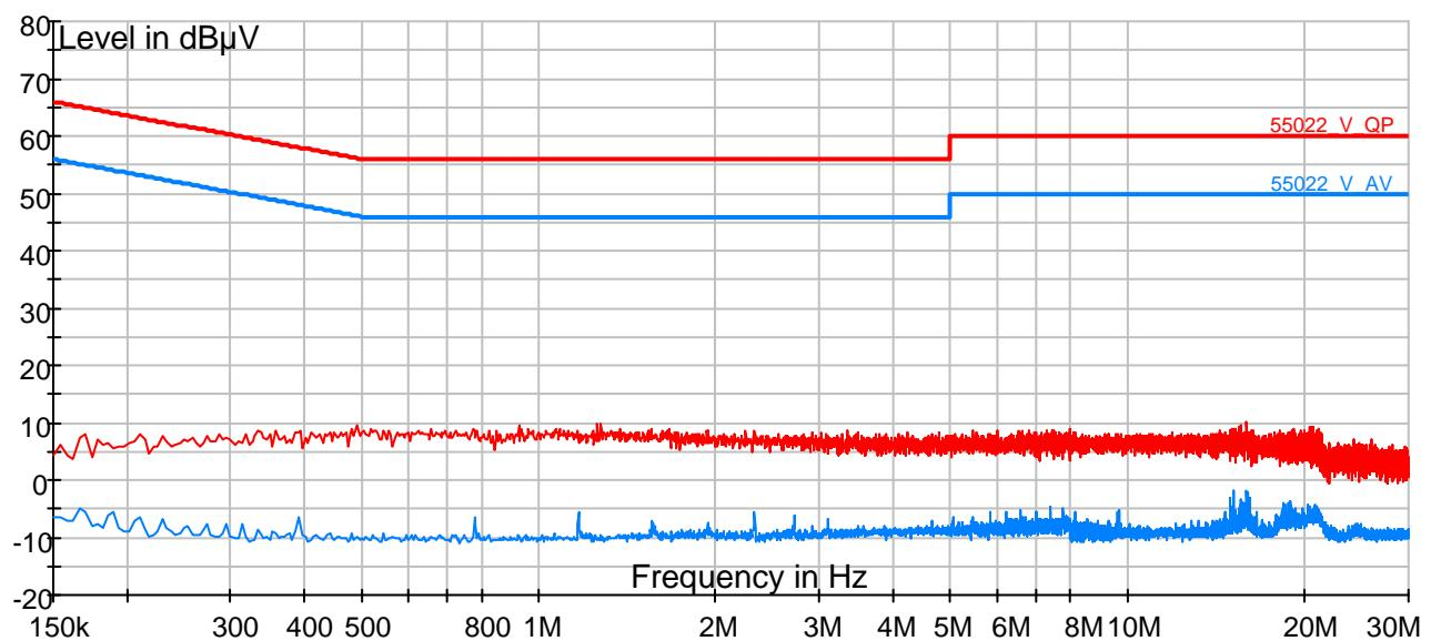
**Port: DC input negative line**
