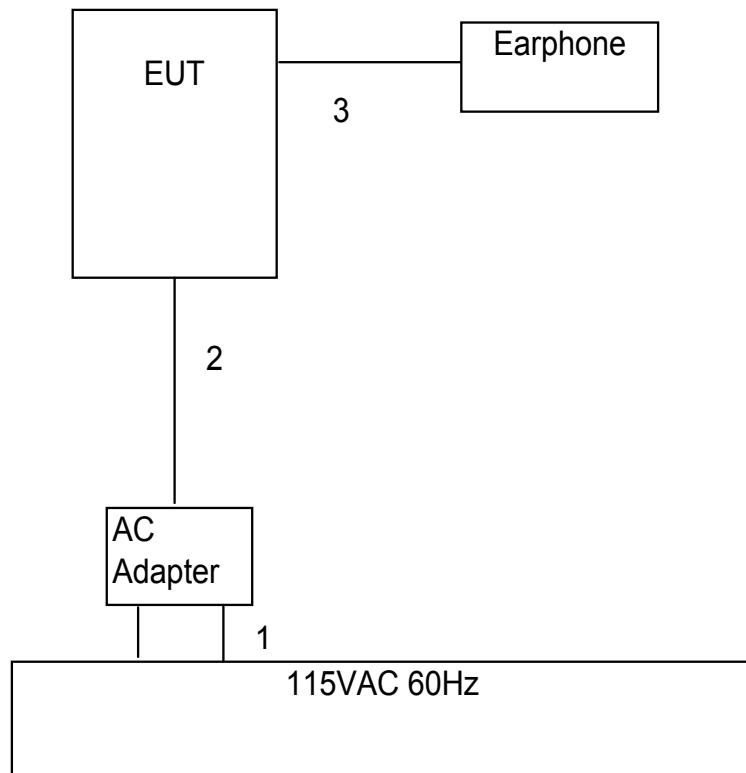
**SETUP DIAGRAM FOR EUT WITH INDUCTIVE CHARGING DOCK**
