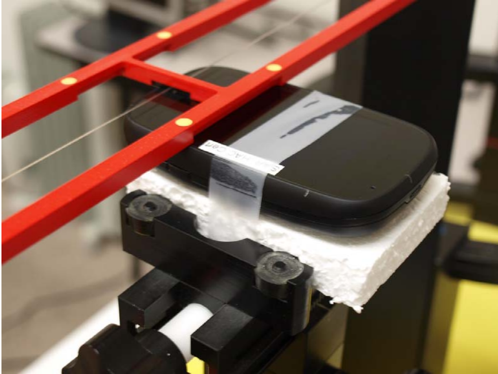
TEST SETUP PHOTO FOR HAC RF EMISSIONS (Slide closed)
