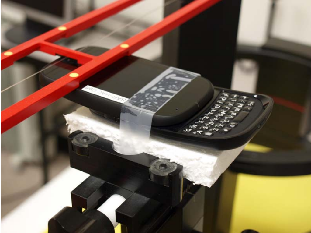
TEST SETUP PHOTO FOR HAC RF EMISSIONS (Slide open)
