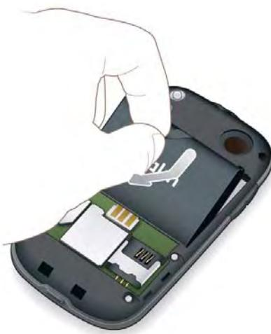
**WARNING** You must remove the battery first whenever you insert or remove the SIM card.
