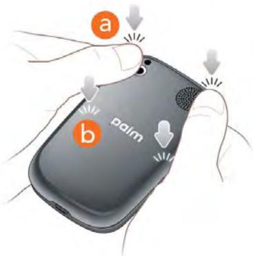
10 Slide out the keyboard (see [Slide out the keyboard](#)), and then press the two snaps at the bottom corners.
