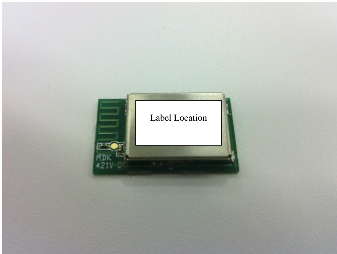
This label drawing image will be directly printed on the shielding case with laser marker.
