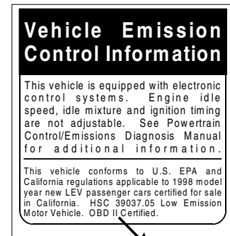
Figure 2. (Right) Vehicle Emission Control Information Label - located inside the hood of most vehicle. Use it to identify whether or not the vehicle is OBD II compliant.
