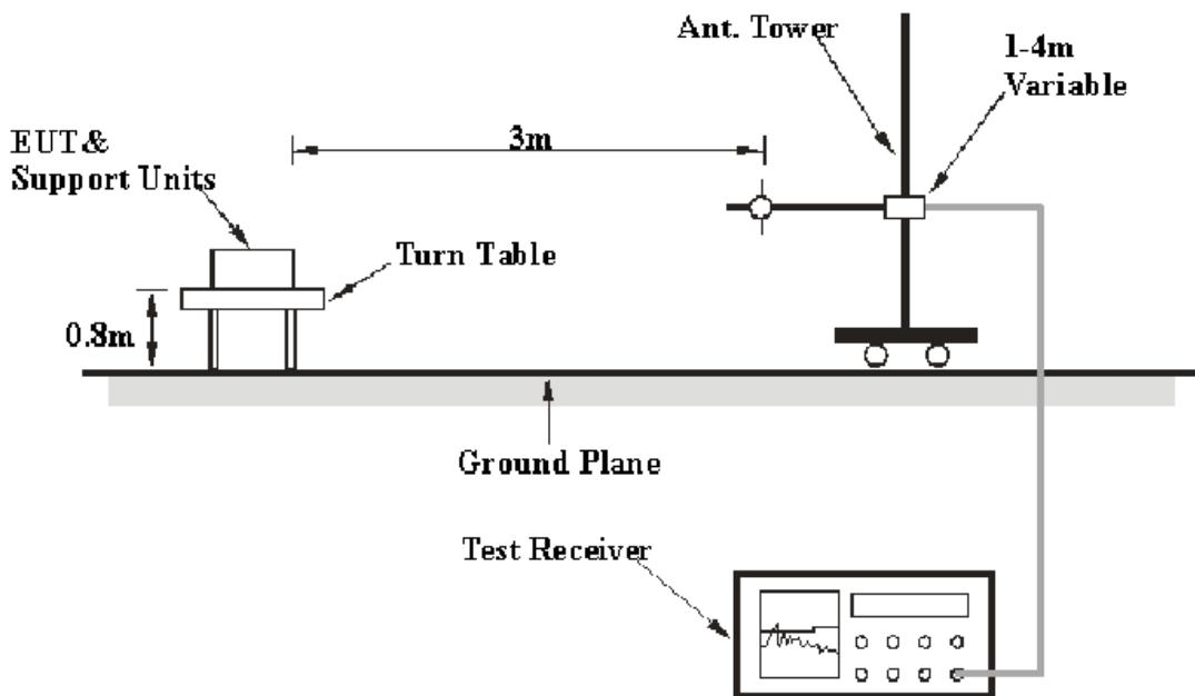
The deactivation test was performed in the 3 meters chamber test site, using the setup accordance with the ANSI C63.4 - 2009. The specification used was the FCC 15.231(a) limits.
