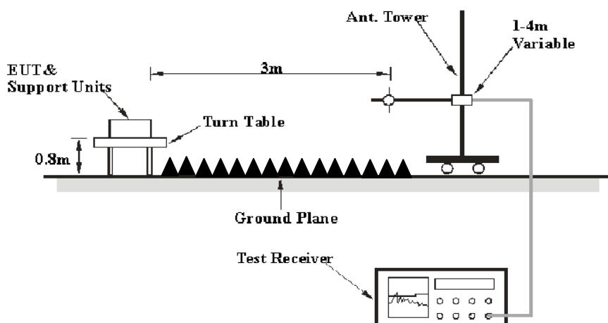
The radiated emission tests were performed in the 3 meters test site, using the setup accordance with the ANSI C63.4 - 2009. The specification used was the FCC 15 § 15.209, 15.205 and 15.231.
