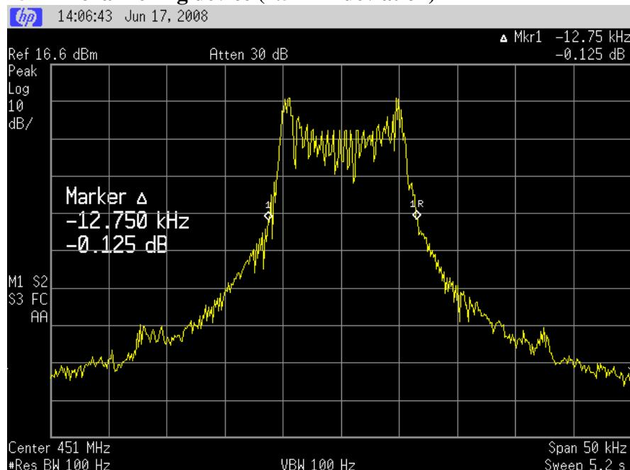
The declared bandwidth has been confirmed even though it is slightly higher than the calculated and measured necessary bandwidth and therefore allows for measurement uncertainties.
