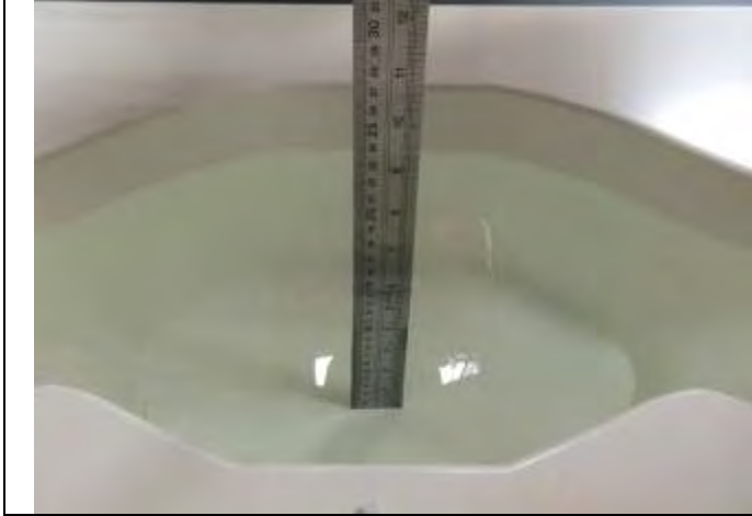
Body Position with 2450MHz liquid depth (15.2cm)
