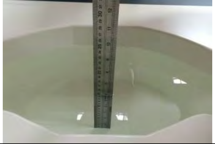
Body Position with 5000MHz liquid depth (15.4cm)
